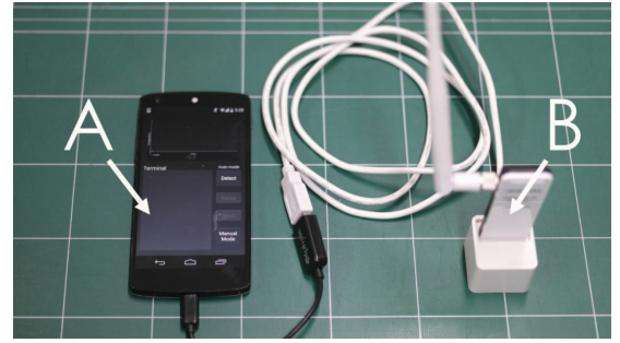
Fig. 9. Hardware setting of the mobile PrAP-Hunter.
